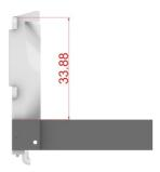
6. Space from front end of frame and front ends of tanks.
