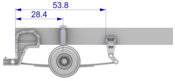
4. Dimensions for front fender's and cab's supports (from front end of frame).
