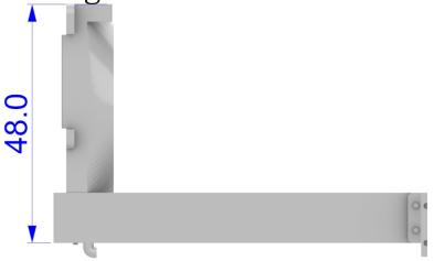
7. Space from front end of frame and front ends of tanks: Left side.
