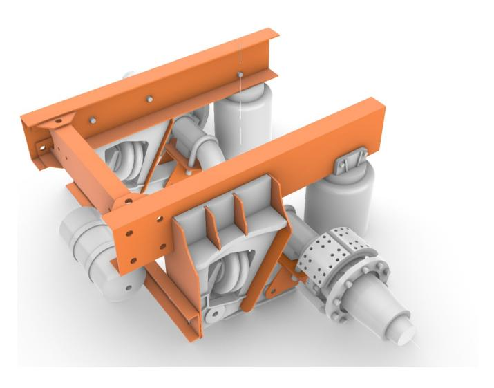
Lift non-steered axle for US trucks Scale, 1/24
