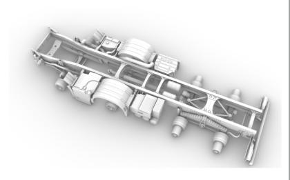
8x4 tandem chassis for Swedish construction truck
